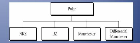
Polar encoding uses two voltage levels (positive and negative).
