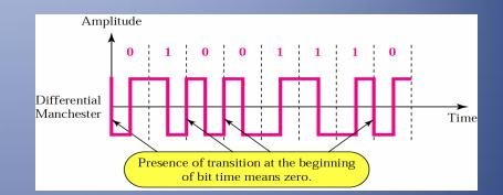
In differential Manchester encoding, the transition at the middle of the bit is used Transition at the middle of the bit is used only for synchronization. The bit representation is defined by the inversion or noninversion at the
