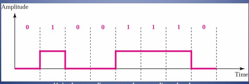
Unipolar encoding uses only one voltage level.
