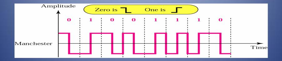
In Manchester encoding, the transition at the middle of the bit is transition at the middle of the bit is used for both synchronization and bit used for both synchronization and bit representation.
